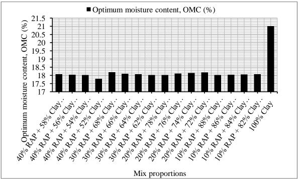
Figure 9 Variation of optimum moisture content (OMC) with various proportions of RAP + Clay + Lime mixes.
