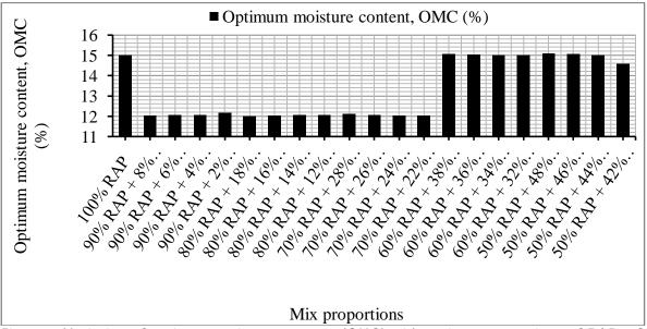
Figure 7 Variation of optimum moisture content (OMC) with various proportions of RAP + Clay + Lime mixes.
