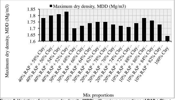
Figure 8 Variation of maximum dry density (MDD) with various proportions of RAP + Clay + Lime mixes.
