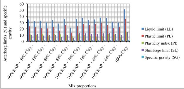
Figure 5 Variation of Atterberg limits and specific gravity with various proportions of RAP + Clay + Lime mixes.
