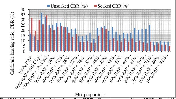
Fig. 10 Variation of california bearing ratios (CBR) with various proportions of RAP + Clay + Lime mixes.
