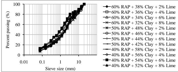
Figure 2 Particle size distribution curves of various proportions of RAP + Clay + Lime mixes
