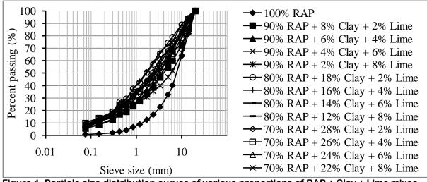
Figure 1 Particle size distribution curves of various proportions of RAP + Clay + Lime mixes
