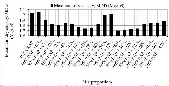
Figure 6 Variation of maximum dry density (MDD) with various proportions of RAP + Clay + Lime mixes.
