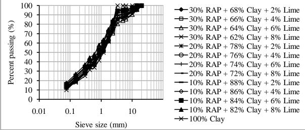
Figure 3 Particle size distribution curves of various proportions of RAP + Clay + Lime mixes
