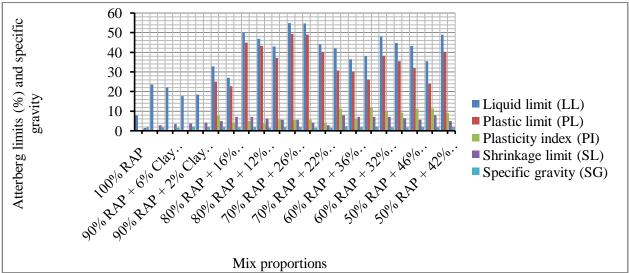
Figure 4 Variation of Atterberg limits and specific gravity with various proportions of RAP + Clay + Lime mixes.
